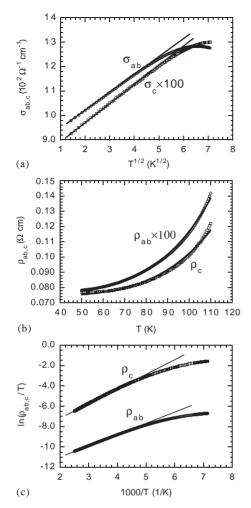
Fig. 1. (a) In-plane conductivity  $\sigma_{ab}$  and out-of-plane conductivity  $\sigma_c$  vs.  $T^{1/2}$  measured down to 1.9 K, (b) in-plane resistivity  $\rho_{ab}$  and out-of-plane resistivity  $\rho_c$  vs. T, (c) plot of  $\ln(\rho_{ab,c}/T)$  vs. 1000/T, for a La<sub>1.2</sub>Sr<sub>1.8</sub>Mn<sub>2</sub>O<sub>7</sub> single crystal measured in zero field.
